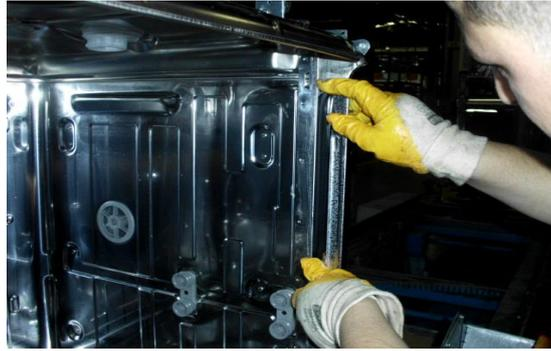
**Figure 2.5.** Assembling the gasket on the inner tube
