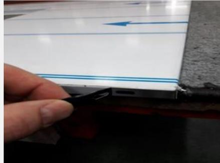
Figure 10: Protective film removal from metal sheet.
