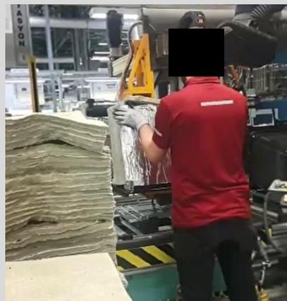
**Figure 2:** Oven insulation installation
