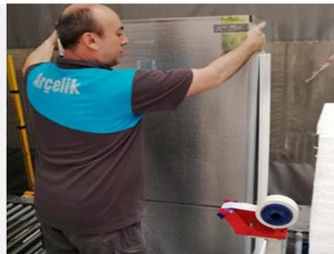
**Figure 5:** Applying the protector to the refrigerator
