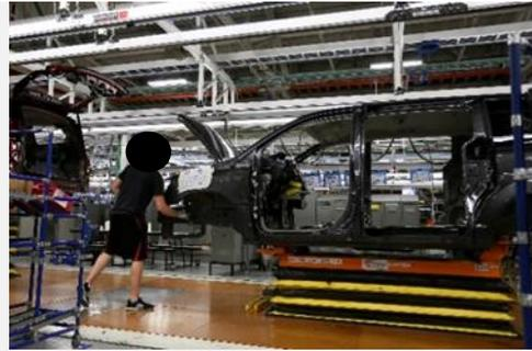
**Figure 15:** Current process in the stop-and-go type
