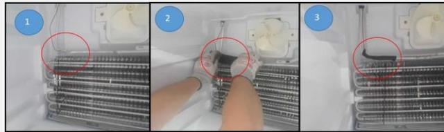
Figure 12: Assembly of bitumen in the refrigerator
