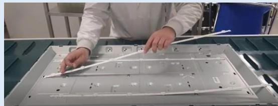
Figure 11: Led bar assembly
