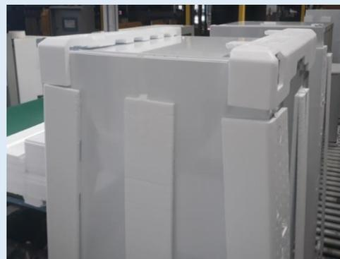
**Figure 9:** Styrofoam Placed Refrigerator
