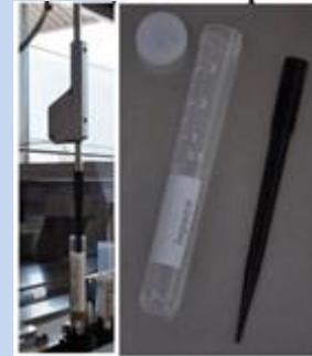
Figure 2: Pipetting unit and tube and tip
